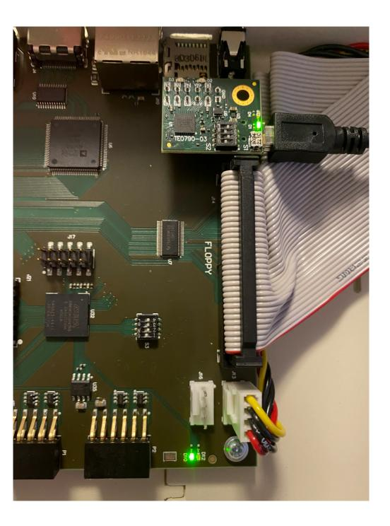
On the PCB R2 MEGA65 mainboard, dip switch 1 (the one nearest to the user sitting in front of the machine) must be in the ON position. The other switches must be OFF. The keyboard will go into "ambulance mode" (blue flashing lights) when set correctly.
